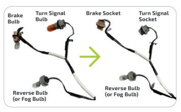
Take out the new tail light. Find the plugs (brake & turn signal plugs) at rear of the new tail light. Connect both plugs to the sockets of harness. Twist all 3 sockets till they are securely connected to the new tail light housing. Please fix the 3 metal fixing plates by a screw driver.
