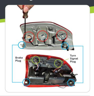
Twist and unlock the 3 bulb sockets to separate them from the tail light housing. Remove the Brake and Turn Signal bulbs from the sockets of harness. Leave the Reverse bulb (or Fog bulb) as it is.
